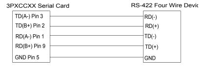
Figure 5. RS-422/RS-485 (Four Wire) Pinout Description
